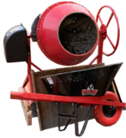
Electric Motor Driven Concrete Mixing Drum. Mixes 4x40kg with 13l water
